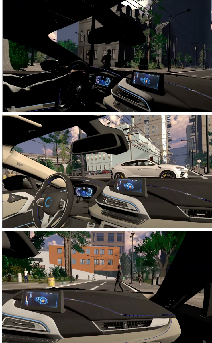
Figure 4.1: Three scripted critical events occurred during the ride from top to bottom: Pedestrians running on the street from left to right, fast cars cutting in the self-driving car path, and pedestrians walking in the middle of the road.
