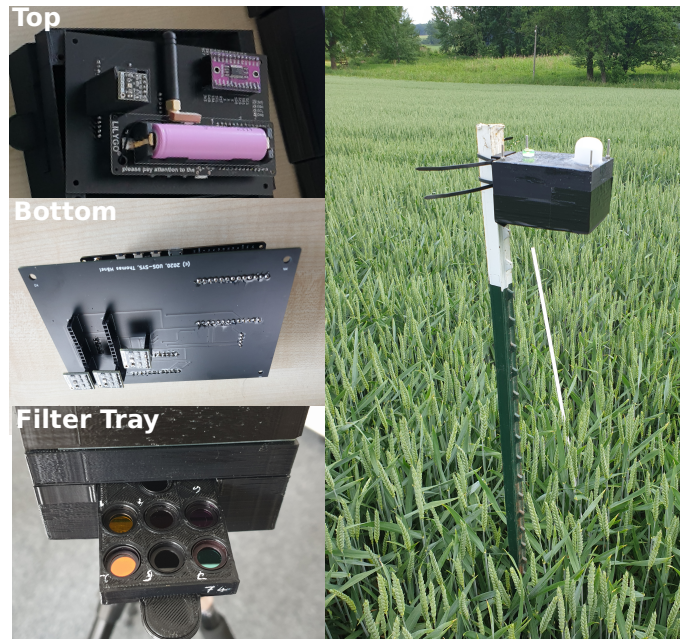
Figure 4.5.: Photos of top and bottom of the connection PCB, the filter tray, and a fully assembled sensor node.
